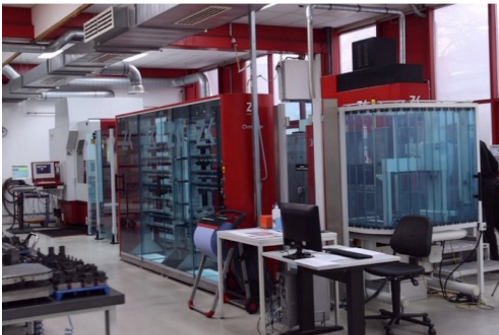
Automation enables unmanned work around the clock, even on weekends. The Zeiss Vista is positioned in the foreground, at the front of the system.
