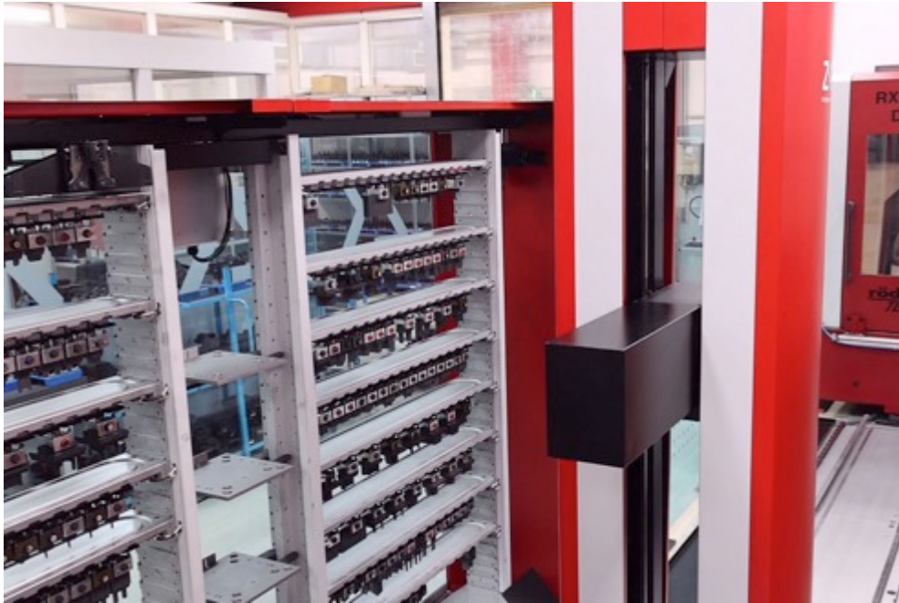
At SD Formentchnik, the Chameleon from Zimmer & Kreim links two genius EDM systems of different sizes with a Rödgers HSC milling machine for electrode machining and a Zeiss Vista measuring machine.
